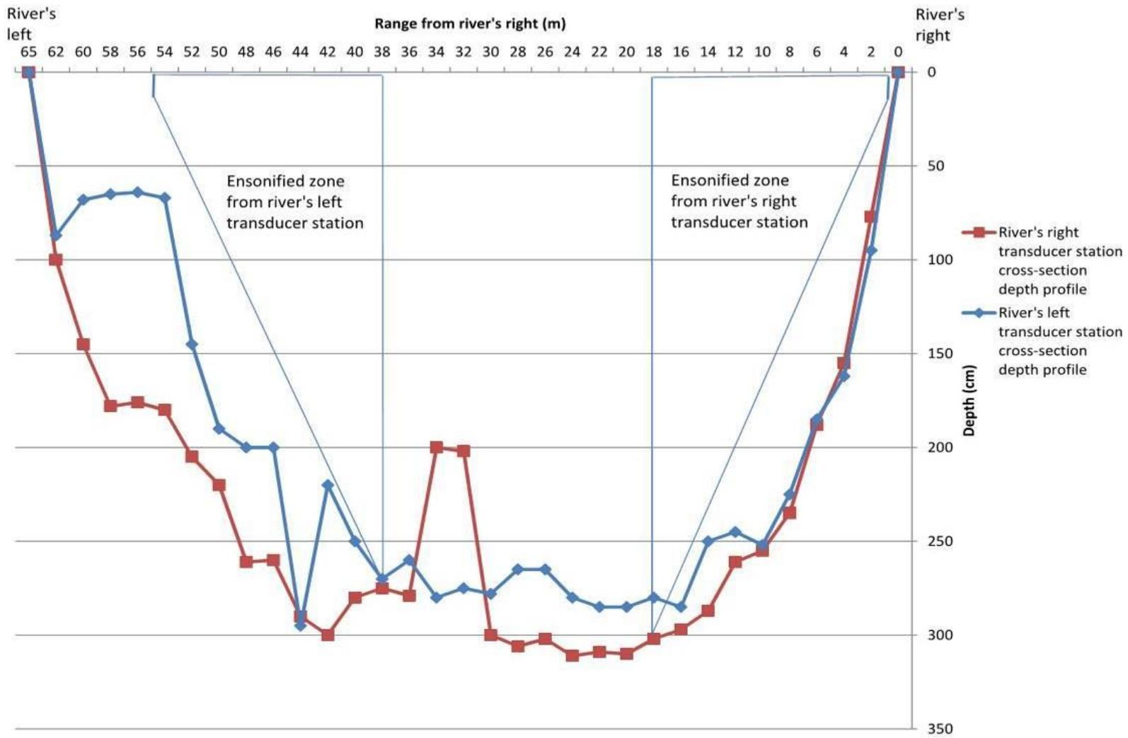
**Figure 7.** Graph showing the Babine River channel cross-sections depth profiles at the two transducer stations located at the Nilkitkwa Lake outlet, and the approximate ensonified zones.
